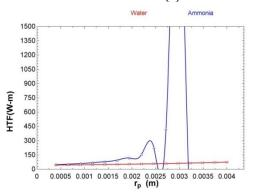
Fig: 13: Plot between HTF and Pore Radius for Ammonia and Water [8]
