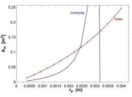
Fig: 12: Plot between Wick Area and Pore Radius for Ammonia and Water [8]
