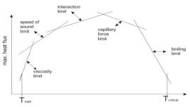
Fig: 3. Limitations of a Heat Pipe [2]
