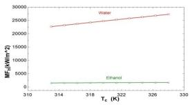
**Fig: 4.** Variation of Figure of Merit and Heat pipe temperature for Water and Ethanol<sup>[8]</sup>
