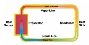
Fig: 1. Circular Process of a Heat Pipe [2]
