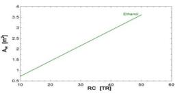
Fig: 8: Variation of Wick area with refrigerating capacity for Ethanol [8]
