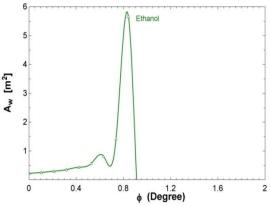
Fig: 9: Variation of Wick Area with Inclination Angle for Ethanol [8]
