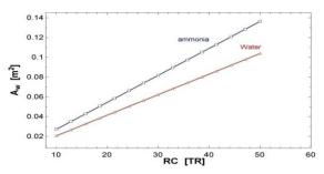
Fig: 7. Variation of Wick area with refrigerating capacity for Ammonia and Water [8]
