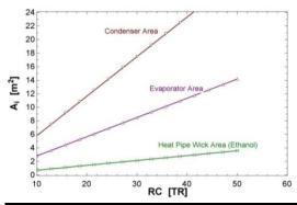
Fig: 15: Variation of condenser, evaporator and wick area with refrigerating capacity<sup>[8]</sup>
